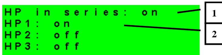
A screenshot of a terminal-style menu for heat pump control. The text is as follows: "HP in series: on", "HP1: on", "HP2: off", "HP3: off". Two callout boxes are present: box 1 points to "HP in series: on" and box 2 points to "HP1: on".
