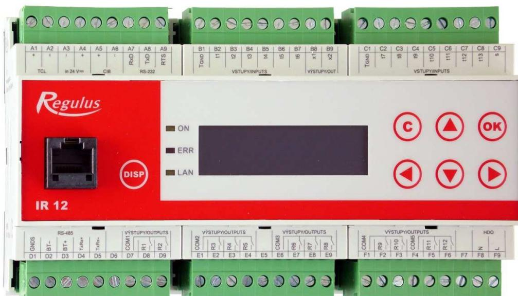
The keys **▲**, **▼** are used to browse in the menu. In order to edit a parameter, press **OK** and a cursor appears on the parameter. The values of numeric parameters can be increased/decreased by pressing **▲** / **▼** keys. Selection parameters (e.g. ON/OFF) are chosen by pressing keys **◀**, **▶**. When finished, pressing **OK** will move the cursor to the next parameter in the same display. Parameter editing can be also exited without saving by pressing the key **C**.
