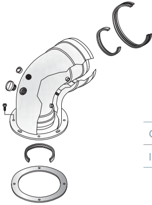
90° flanged elbow ø 60/100 with tap holes
