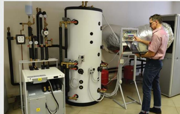
Pressure testing of thermal stores
