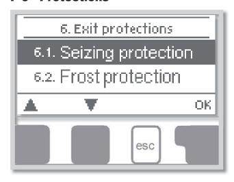
Menu "6. Protections" can be used to activate and set various protective functions.
