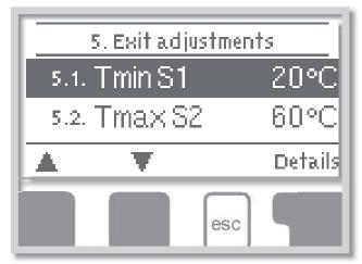
The necessary basic settings required for the control function are made in menu "5. Settings".
