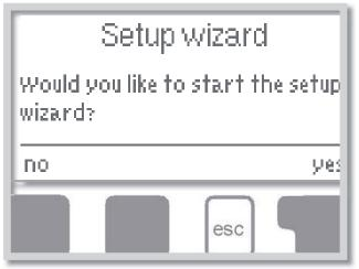
The first time the controller is turned on and after the language and time are set, a query appears as to whether you want to parameterize the controller using the commissioning help or not. The commissioning help can also be terminated or called up again at any time in the special functions menu. The commissioning help guides you through the necessary basic settings in the correct order, and provides brief descriptions of each parameter in the display.
